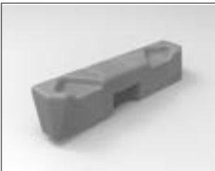
Soundproofing of the central pillar of the body, lower
